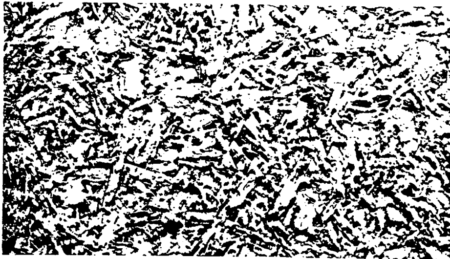
Figure 5. Plutonium-39 a/o carbon alloy, heat treated at 555°C for 864 hr. 500 X. Zeta blades in a matrix of alpha plutonium.
